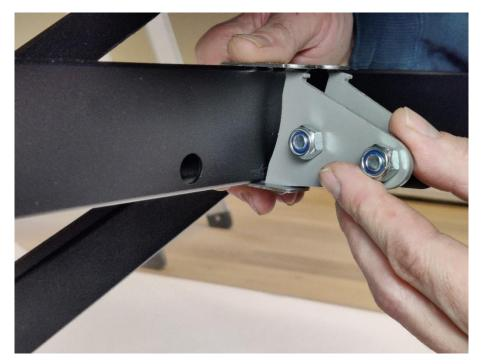
Press the stainless-steel mounting bracket closed so that the side plates hook into the slots of the mounting bracket.
