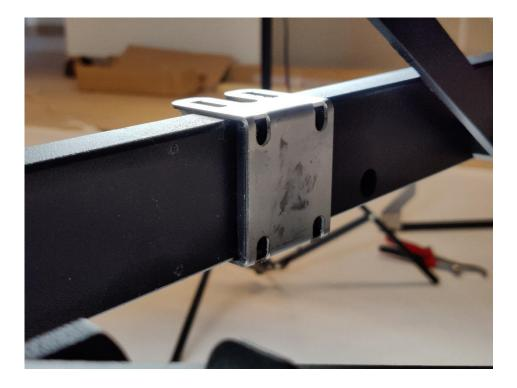
Tighten the screws to secure the clamp to the frame.
