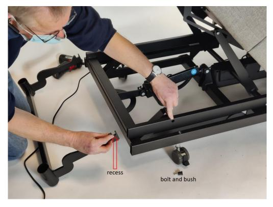
Replace bolt and bush on both sides of the frame.
