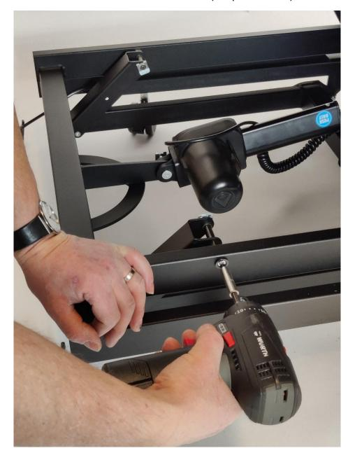
Slide the bracket as deep as possible into the frame.
