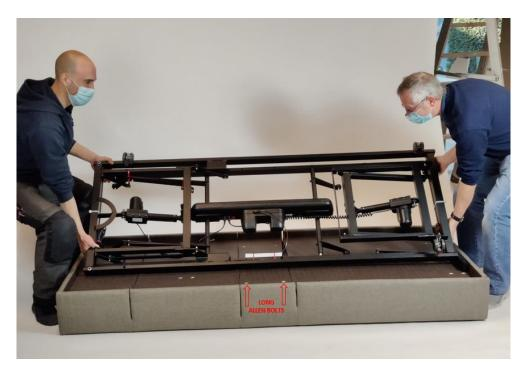
Remove all red cable ties, including those securing the mains cable and the remote control.
