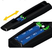
Once the batteries have been inserted, close the battery compartment lid again and the radio remote control is operational.
